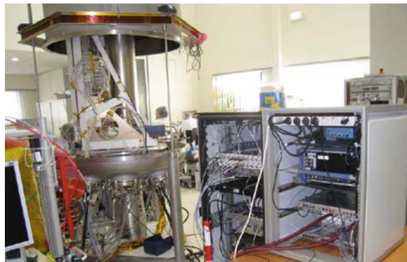
Figure 3: ACES EM system level tests at the CNES facilities in Toulouse. On the left, the vacuum chamber with the ACES EM workbench before being closed; the PHARAO tube is also visible. On the right, the RF support equipment and part of the measurement instrumentation.
